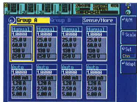
Range setting and scaling
