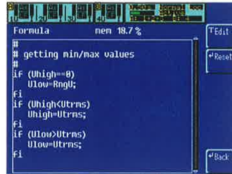
Program example for the monitoring of overvoltage and undervoltage
