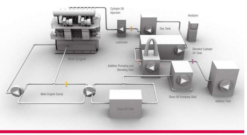
Fig. 1: Drawing of the SEA-Mate® B2000 Blending
